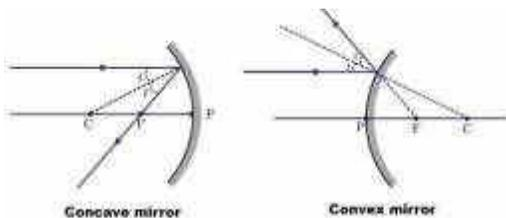
(ii) A ray passing through the principal focus of a spherical mirror, after reflection, will emerge parallel to the principal axis.
