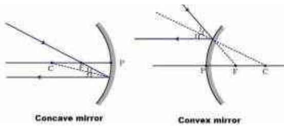
**(iii) A ray passing through the center of curvature of a spherical mirror, after reflection, is reflected back along the same path.**
