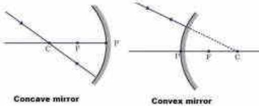
**(iv) A ray incident obliquely to the principal axis is reflected obliquely following the laws of reflection, i.e., angle of incidence is equal to angle of reflection.**
