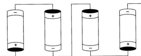
**Ans 4.** The problem in this circuit is the improper connection of two cells. In the circuit positive terminal of one cell should be connected with negative terminal of other to make the bulb glow as given in the figure.
