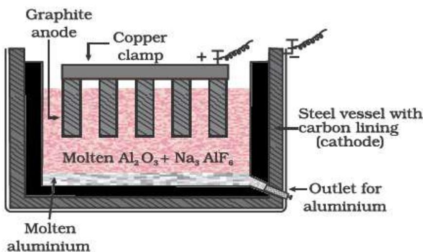
The addition of cryolite ( $\text{Na}_3\text{AlF}_6$ ) and fluorspar ( $\text{CaF}_2$ ) makes alumina a good conductor of electricity and lowers its Fusion temperature from 2323 to 1140 K. the reaction taking place
